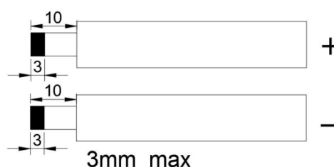
Fig.12 Schematic diagram of AC input/output connection
