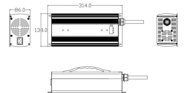
Tolerance of outline dimension is  $\pm 0.5$  mm, others are  $\pm 0.2$  mm in the diagram
